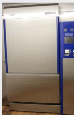
The autoclave sterilizes medical waste from a patient and personal protective equipment worn by staff.
